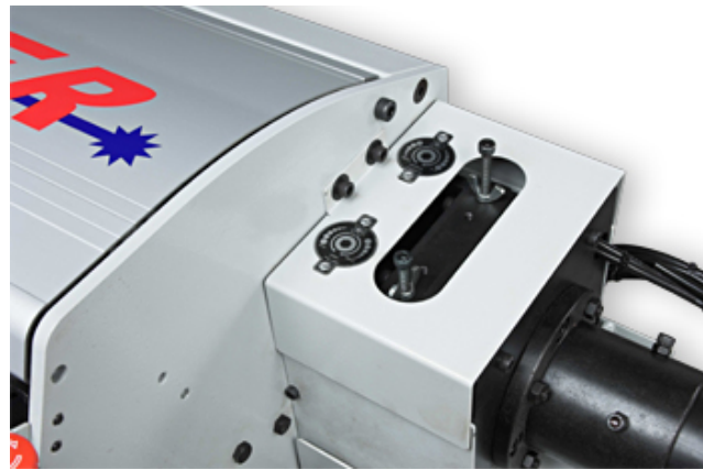
Connected SteadyRest -Anti-Vibration device
