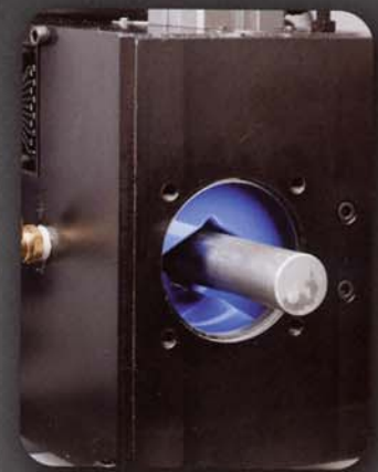
Simple adjusting "V" type anti-vibration device, no changeover required.
